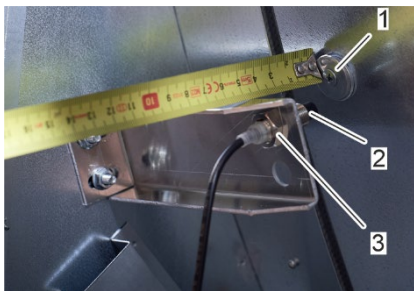
Fig. 77: Adjust clock sensor
