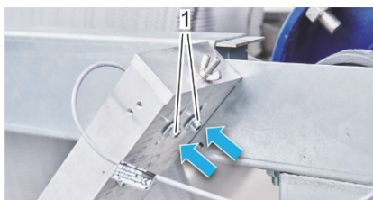
Fig. 32: Screws of the deflector roll
