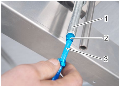
Fig. 61: push compressed air hose in compressed air nozzle
